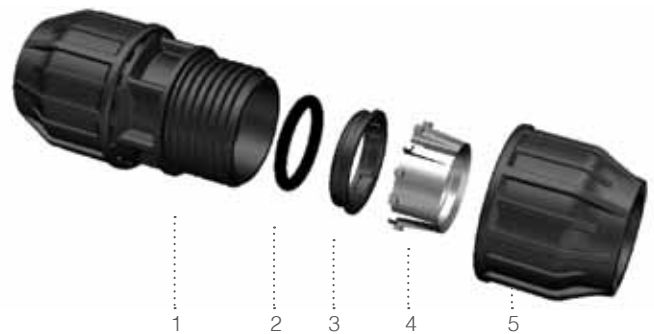
1. BODY - Polypropylene PP-B / 2. O-RING - Nitrile Rubber (NBR 70) / 3. INSERT - Polypropylene PP-B / 4. SPLIT RING - Polyacetal / 5. NUT - Polypropylene PP-B
